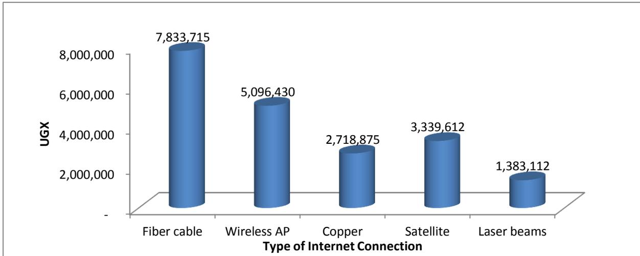
The graph above shows the average cost of bandwidth per month by type of internet connection in MDAs. The highest average cost per month of bandwidth (7.8m) across most MDAs is delivered through fiber cable. This is followed by wireless, copper, satellite and laser beams with 5m, 2.7m, 3.3m and 1.3m respectively.
